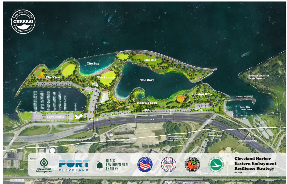
A plan view of the Cleveland lakefront CHEERS project, Cleveland Harbor Eastern Embayment Resilience Strategy, shows a reconfigured park made of landfill with larger sheltered bay and cove areas designed to withstand wind and wave action.
